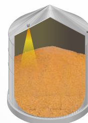
Ultrasonic level meter
