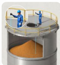
Laser distance measurement
