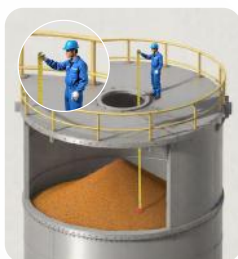
Plumb line measurement
